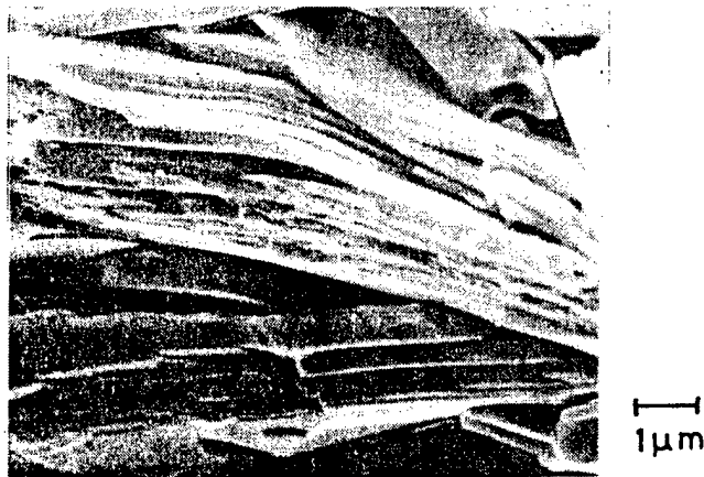
Figure 2. SEM Image of Tape Wire Ruptured Surface
