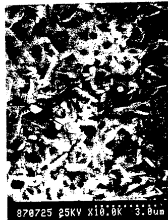
Fig.6 SEM photograph of a YBCO thin film sputtered at a substrate temperature of 250°C and post annealed in O 2 flow at 900°C for 15 minutes and 450°C for 4 hours
