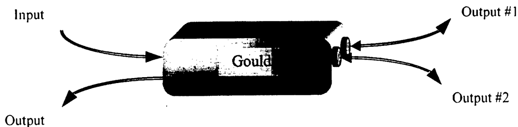
Figure 3.2 Asymmetrical fiber optic coupler illustrating the primary input and output ports. Note that Output ports #1 and #2 serve a dual function (refer to text).
