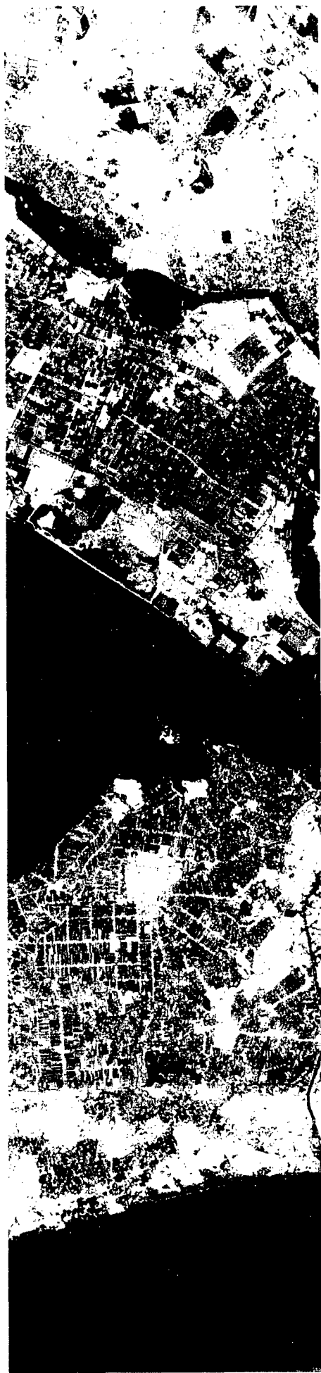
Space borne polarimetric image (SIRC, 5.3 cm) RGB: HH/HV/VV
