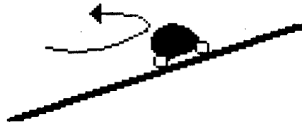
Figure 5: A circular automobile racetrack is banked at an angle of 20 degrees and no friction between road and tires is required when a car travels at a certain speed. If the radius of the track is 400m, determine the velocity.
