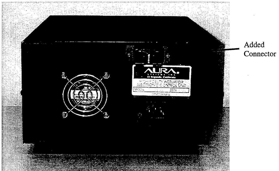
Figure 4.8. ECU rear cover with an added speaker-type push connector
