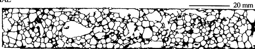
Fig. 1: Image scan of optical micrograph of foamed AlMg1Si0.6 plate ( \rho^*/\rho_s = 0.2 ).
