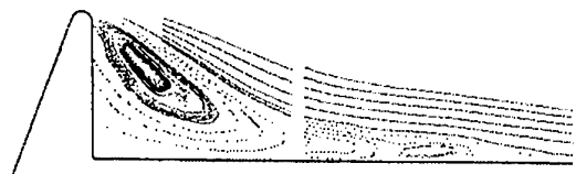
Fig. 13 HEG run 132 particle paths from DSMC computations
