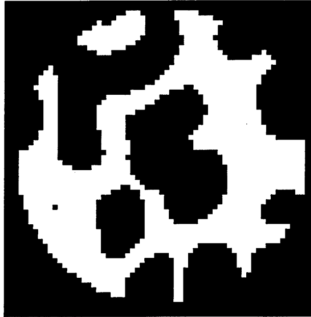
Fig. 1: Sample VGP pupil function. White indicates low-curvature regions. Note the telescope secondary obscuration is not readily apparent because it is contiguous with two regions of high wavefront curvature, which are masked by this realization of the VGP pupil function.
