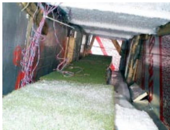
Figure 1. FERG frosting apparatus. Untreated, frosted turf is in the foreground and FROST-B-GONE-treated turf is in the background.
