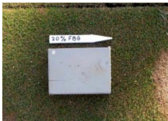
Figure 2. Wooden block used to compress turf to cause injury after frosting.
