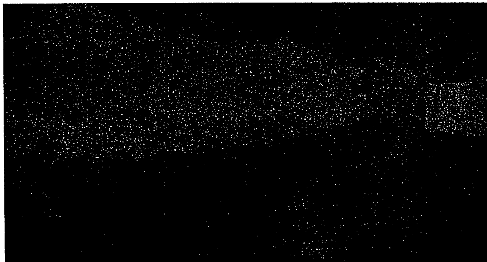
Figure 6. Shearogram of Hot Air Gun Plume 10 Seconds After Heat Element Turned Off
