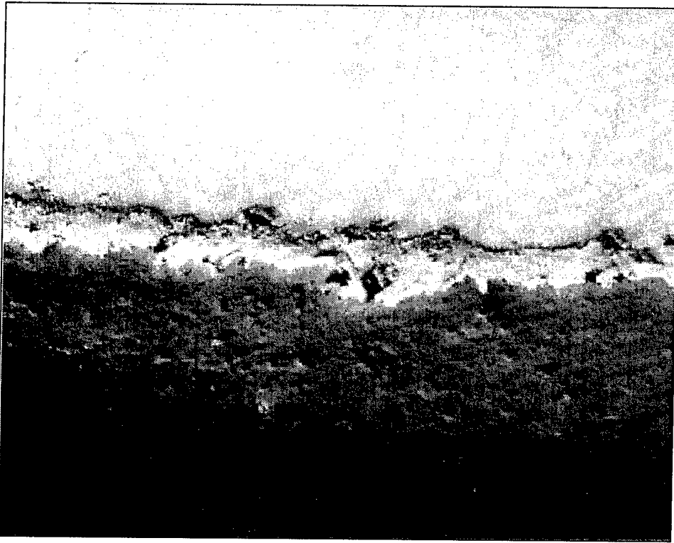
Figure 3. Cross section of alumina-40% titania coating with nickel-chrome interlayer and no seal coat (Specimen 3).
