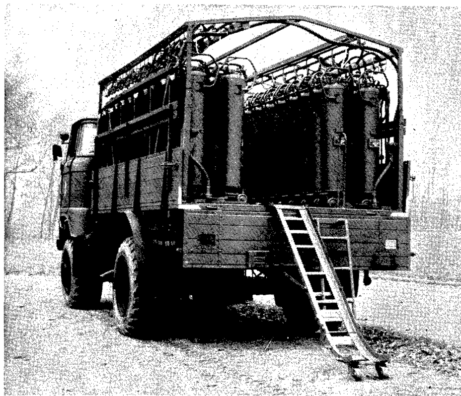
Photo 1. EA 12 special treatment unit (without canvas) with loading ramp and roll-off accessory
