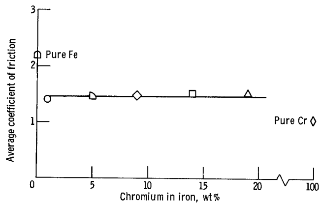
Figure 5. - Average coefficients of friction for iron-chromium alloys, iron, and chromium sliding on themselves. Single pass; sliding velocity, 3 mm/min; load, 0.05 to 0.4 N (5 to 40 g) for alloys, and 0.2 N (20 g) for iron and chromium; room temperature; vacuum pressure, 10^{-8} pascal. (Data from figs. 3 and 4.)
