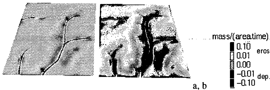
Figure 2. Change in the magnitude of erosion/deposition with C = 1 and increase in both Kt and Kd ;
