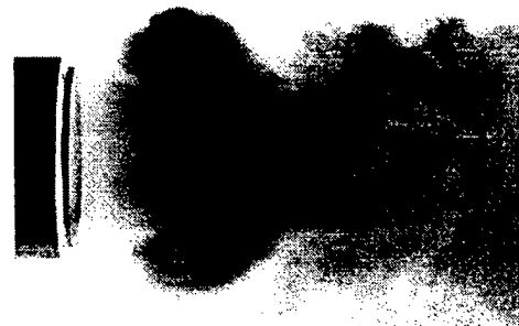
Fig. 2 Planar Mie scattering image of the coherent vortex produced in the larger scale dump combustor incinerator via acoustic forcing; flow is left to right.
