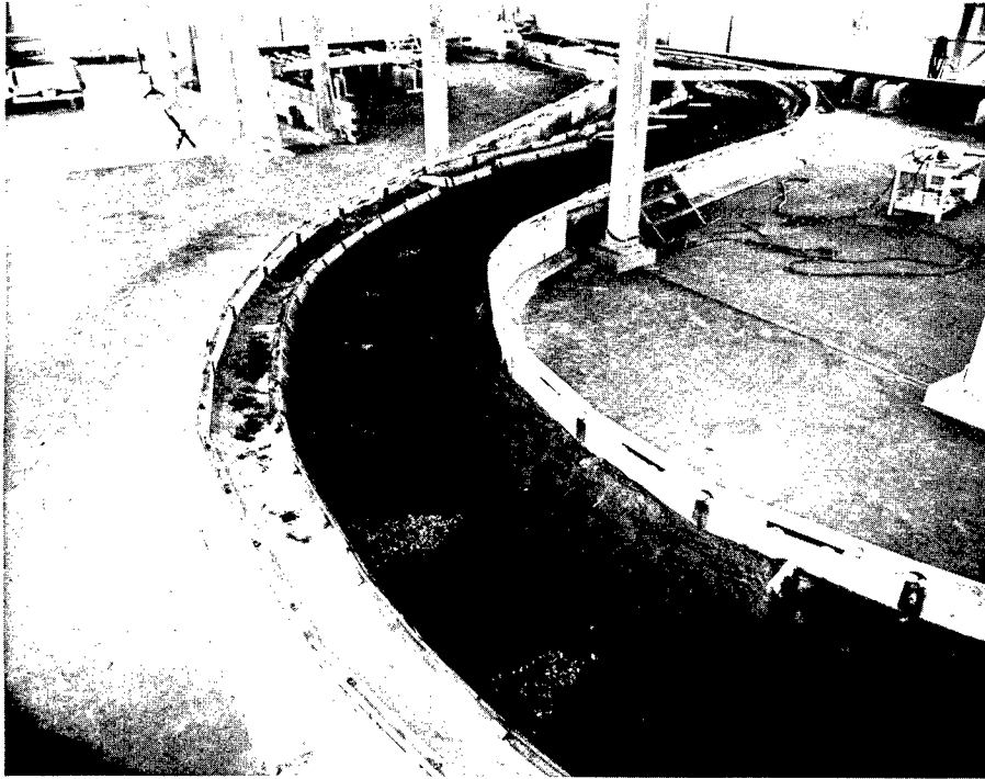
Figure 8 - Photograph of Model Bed at Completion of Test Using low elevation concave bank sills.
