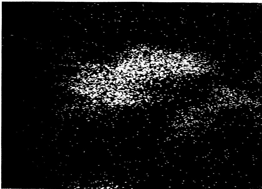
(b) Iron K_{\alpha} X-ray map of silicon carbide; 5.5 \times 10^3 counts.
