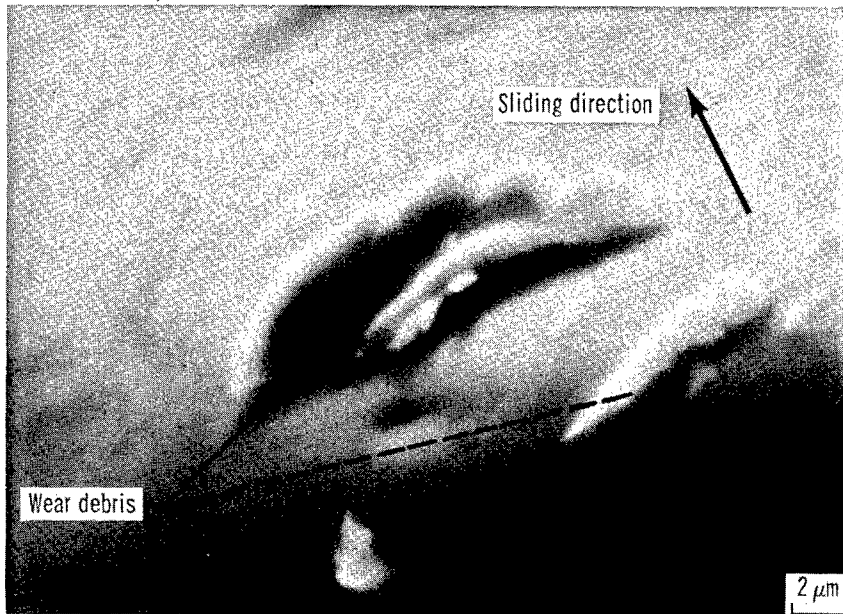
(a) Iron wear debris transferred to silicon carbide.
