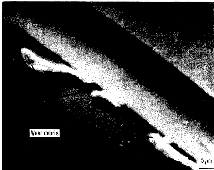
Figure 4. - Iron wear debris and grooves on iron surface. Single-pass sliding of 0.04-millimeter-radius silicon carbide rider; sliding velocity, 3 mm/min; load, 25 grams (0.25 N); temperature, 25° C; environment, argon; pressure, atmospheric.
