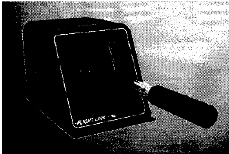
Figure 5-5. The Flight Link helicopter collective control.
