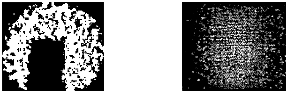
Fig 6: X-ray fields at 30 cms from output of the prototype optics I (left) and II (right). (The blur is a cause for concern for resolution properties).
