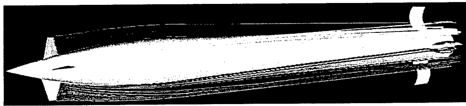
b. Particle traces for Mach 2.2, 0^\circ angle of attack.
