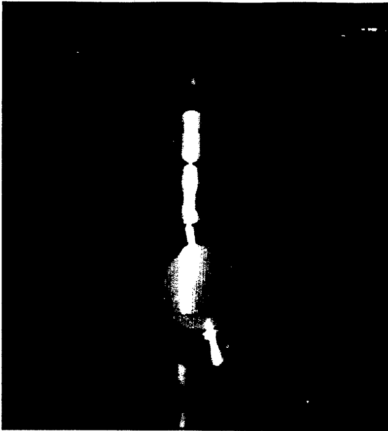
Figure 3.5 A vortex stabilized 915MHz driven air discharge in a resonant cavity. Note plasma jet emerging from the top.
