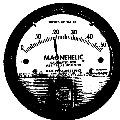
Figure A-44. Magnehelic Gauge. Courtesy Dwyer Instruments, Inc.
