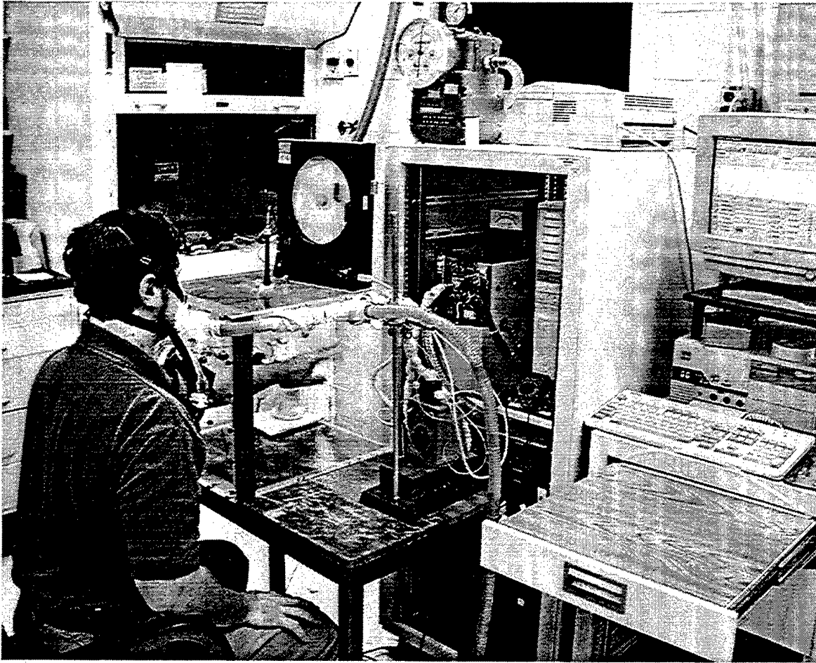
Figure 3-1. Photograph showing subject with arm inserted into Plexiglas chamber containing solvent vapor. Subject is fitted with face mask, one side of which is attached to purified air supply; outlet carries exhaled breath sample to real-time breath analyzer.
