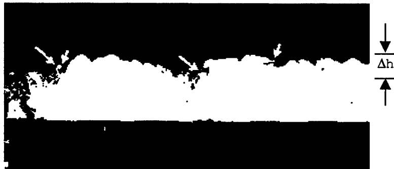
Figure 1 Depiction of the Entrainment Zone in a Convection Tank, from Deardorff et al. (1979). Light areas show the well mixed fluid. The region indicated by \Delta h is defined as the entrainment zone.
