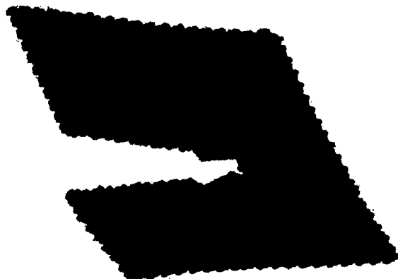
Figure 5: Molecular statics configuration for a loading of twice the Griffith value.
