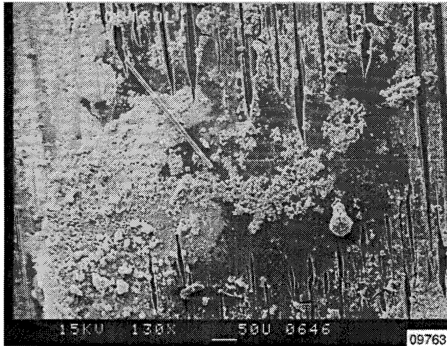
B) THE CONTROL SAMPLE CORRODED FOR 48 HR, VIEWED IN A REGION WELL BELOW THE SALTWATER-JET FUEL INTERFACE. NOTE THE EXTENSIVE MICROCRACKING OF THE RESIN
