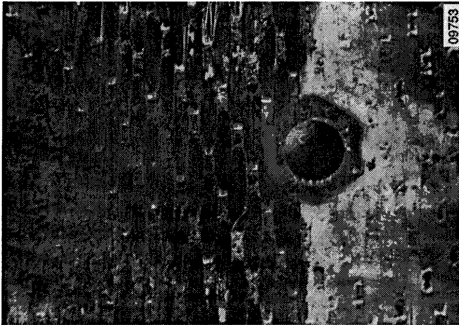
Figure 10c. Close-up view of a Matrimid 5292 sample corroded 96 hr at 80°C
