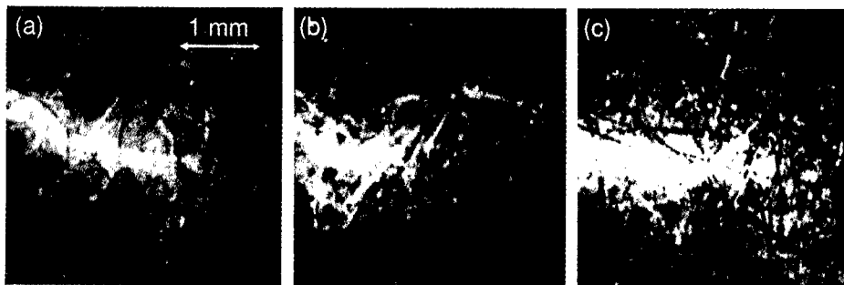
Figure 4. Damage shown with the light shades of gray in mixtures of PGW and softwood kraft (black) in SENT. The mass fraction of kraft fibers is 5% (a), 10% (b) and 20% (c).
