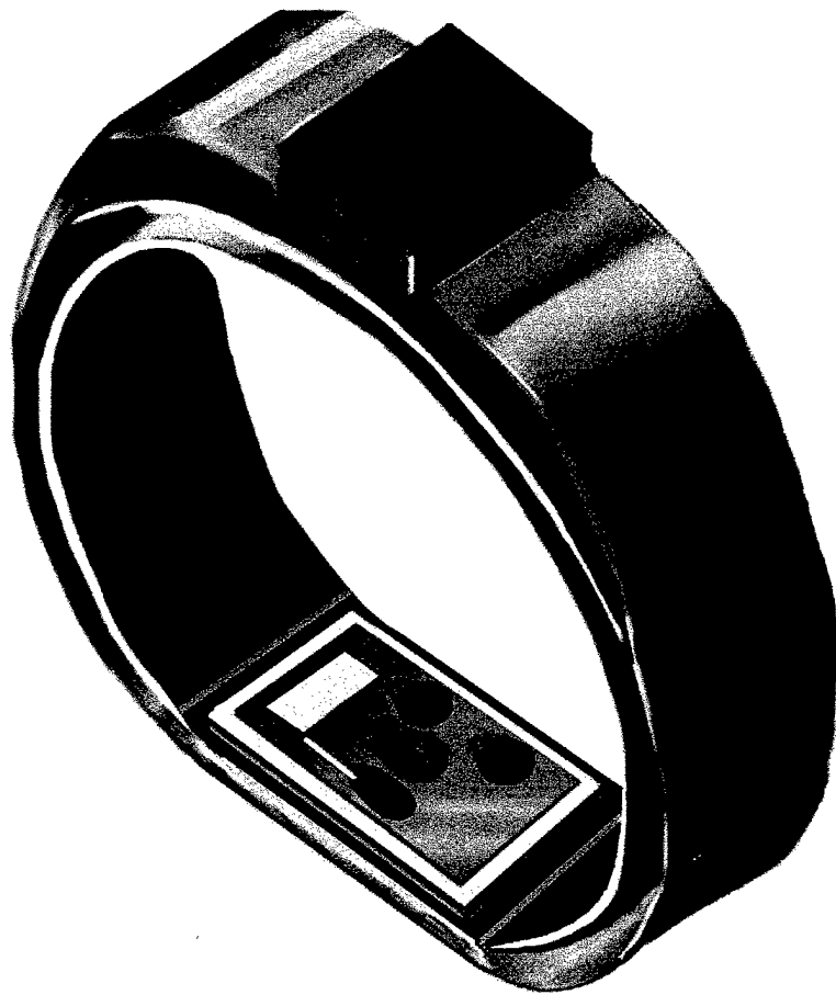
Figure 4.10. Wireless Pulse-Oximeter Finger Ring. Three light-emitting diodes are shown in the bottom portions as the circular reddish portions. One of the light-emitting diodes provides a reference for the distance to the photodiode detector. The two signal-producing sources are sequentially lit by the electronics shown as the gray rectangular region. A duty-cycle receiver/controller appears as a dark oval connected to the other electronics by the yellow segment. The "stone" in the ring is a lithium-ion battery and the ring itself is an antenna and contains a wire bundle. Under the battery at the top of the ring is a photodiode detector, pre-amplifier, and the beta-model telesensor ASIC, including the crystal. The ring has a flexible fit and leaf springs to reduce motion artifacts which are further reduced by digital adaptive filters referenced to the auxiliary source. Comparison of the light absorbed at 670 nm and 780 nm produces the oxygen saturation level. The 780 nm source is used to track the pulse and its transmission is insensitive to skin color.
