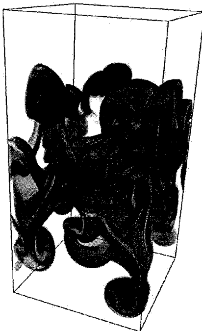
FIG. 3 Rayleigh-Taylor flow: \rho_1/\rho_2 = 3 . \rho = 2\rho_2 isosurface at t = 3.54 . Neighboring- \rho isosurfaces rendered transparent.
