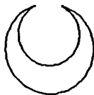
Figure 4.17 Schematic of pinhole formation and a route to deviation from wall thickness uniformity
