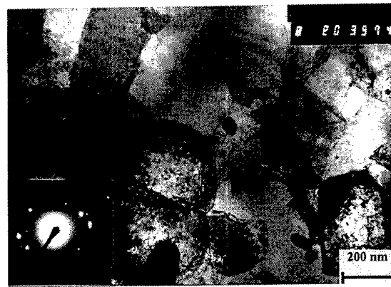
Fig. 9. Microstructure and SAED pattern after ECA pressing.
