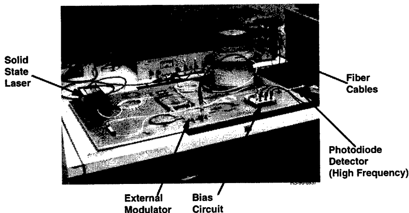
Figure 5. Photo of Optic Link Showing Components of Block Diagram
