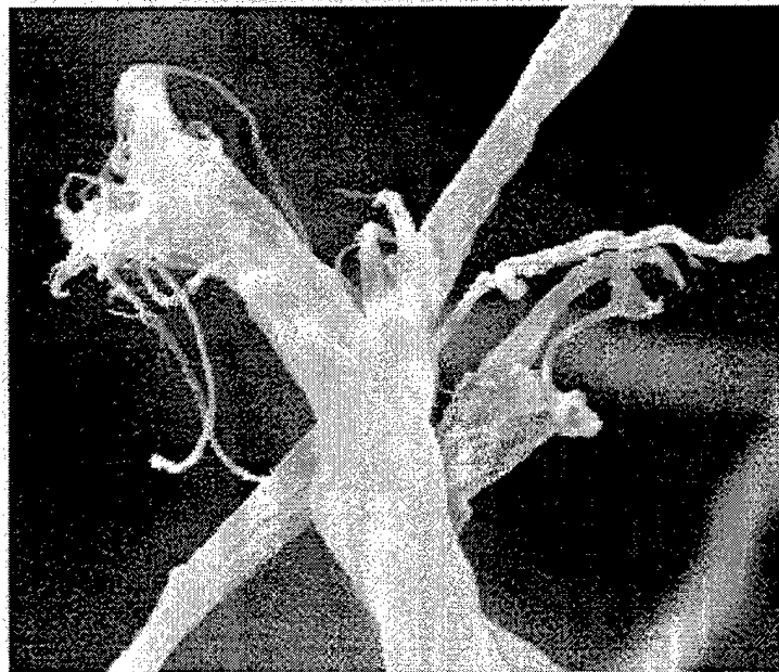
FIGURE 14. FIBERS FROM WOVEN KEVLAR FABRIC (AFTER FAILURE IN YARN TENSILE TEST)
