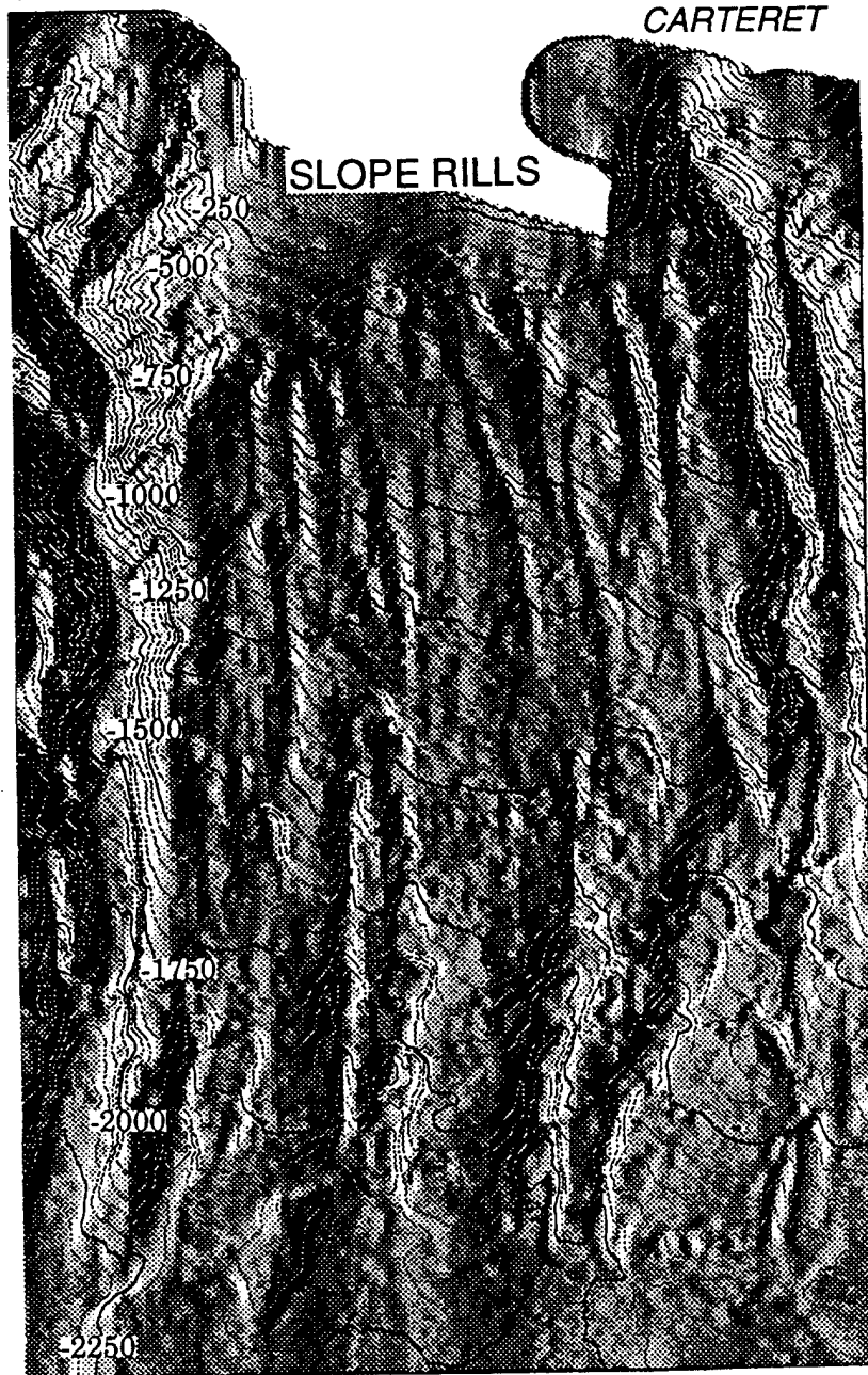
Figure 4. Close-up of slope rills on the intercanion divide between Linden Kohl (left) and Carteret (right) Canyons. Contours show that approximately 11 rills, each on average 20–40 m deep and 300 m wide, initiate on the upper slope at 250- to 500-m water depth. The rills join one another downslope forming several rill networks that enter into three lower-slope, box-shaped canyons that are more than 100 m deep and a kilometer wide.
