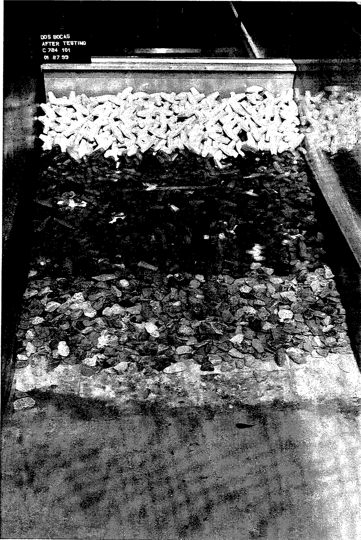
Photo 92. Repeat test of Plan 5. Sea-side view after attack of 7-m waves
