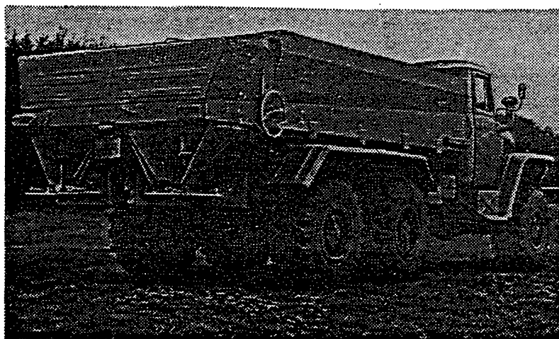
The Ural-5557 with equipment for spreading mineral fertilizers
