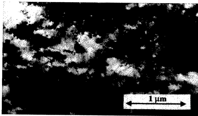
Figure 3: Plan view TEM micrograph showing threading dislocations in the InAs epilayer
