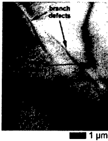
Figure 1. PVTEM image of branch defects in \text{In}_x\text{Ga}_{1-x}\text{P}/\text{GaP} graded to x = 0.26 . The branch defects pin dislocations and sharply turn bend contours.
