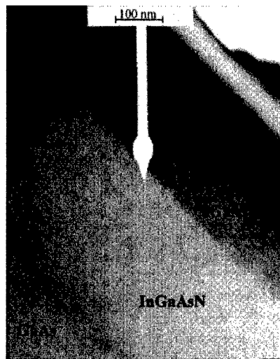
Figure 3. Cross sectional TEM of an as-grown p-InGaAsN showing no sign of dislocations within the resolution limit of 10^7 \text{ cm}^{-2} .
