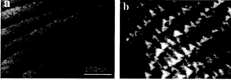
Figure 1: AFM images of 20-nm-thick \text{CaF}_2/\text{Si}(111) . (a) An as-grown surface at 770°C. (b) A surface modified by 2 ML growth at 150°C on the surface shown in Fig. 1(a).
