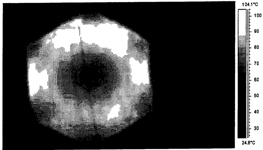
Figure 14. Temperature Profile of Ceramic Tile/Steel Mesh.
