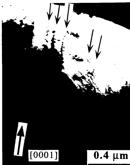
Fig. 5—Bright-field image of a kink boundary showing that it is composed of dislocation walls (indicated by arrows).
