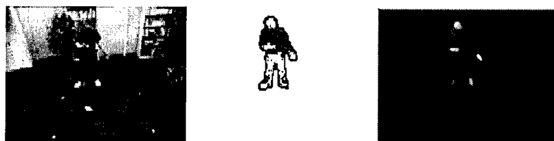
Fig. 4. Analysis of a user in the interactive space. Frame ( left ) is the video input (n.b. color image possibly shown here in greyscale for printing purposes), frame ( center ) shows the segmentation of the user into blobs, and frame ( right ) shows a 3-D model reconstructed from blob statistics alone (with contour shape ignored).
