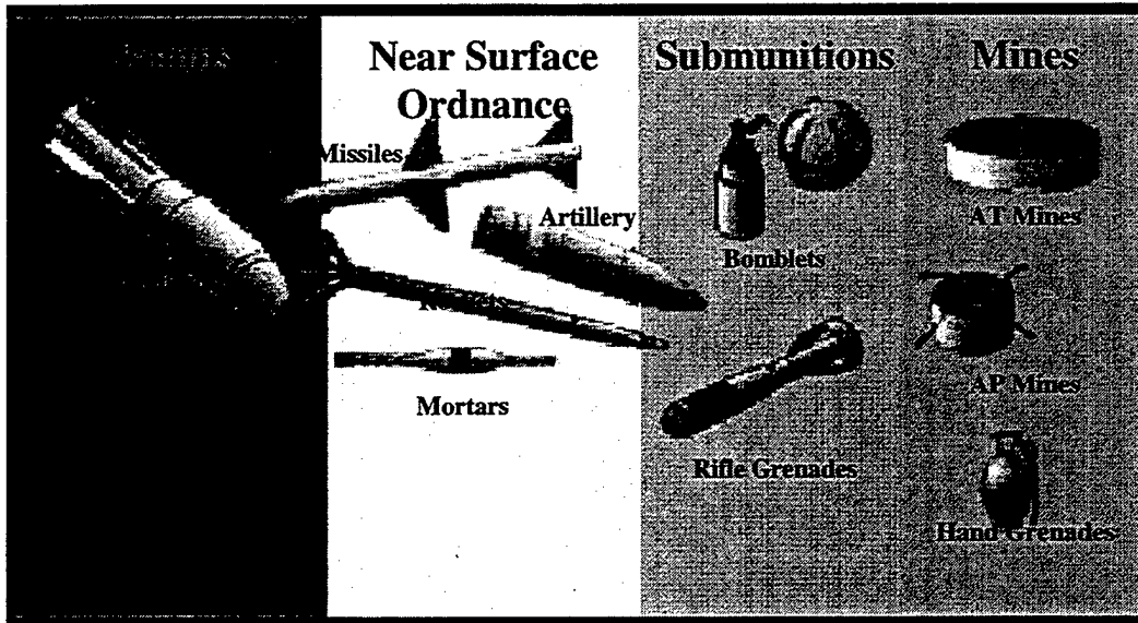
Figure 1: Common Types of UXO and UXO Categories. Different types of UXO impose a varying degree of difficulty for their removal. UXO type is thus an indicator of the cost of UXO removal. From [USD(A&T),1998].
