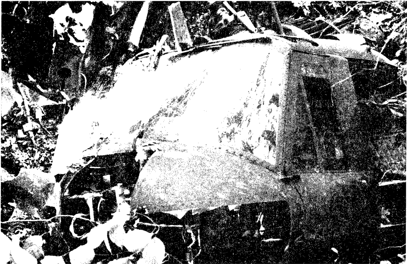
Engine rpm decreased during low-level flight, and UH-1 settled into trees.
