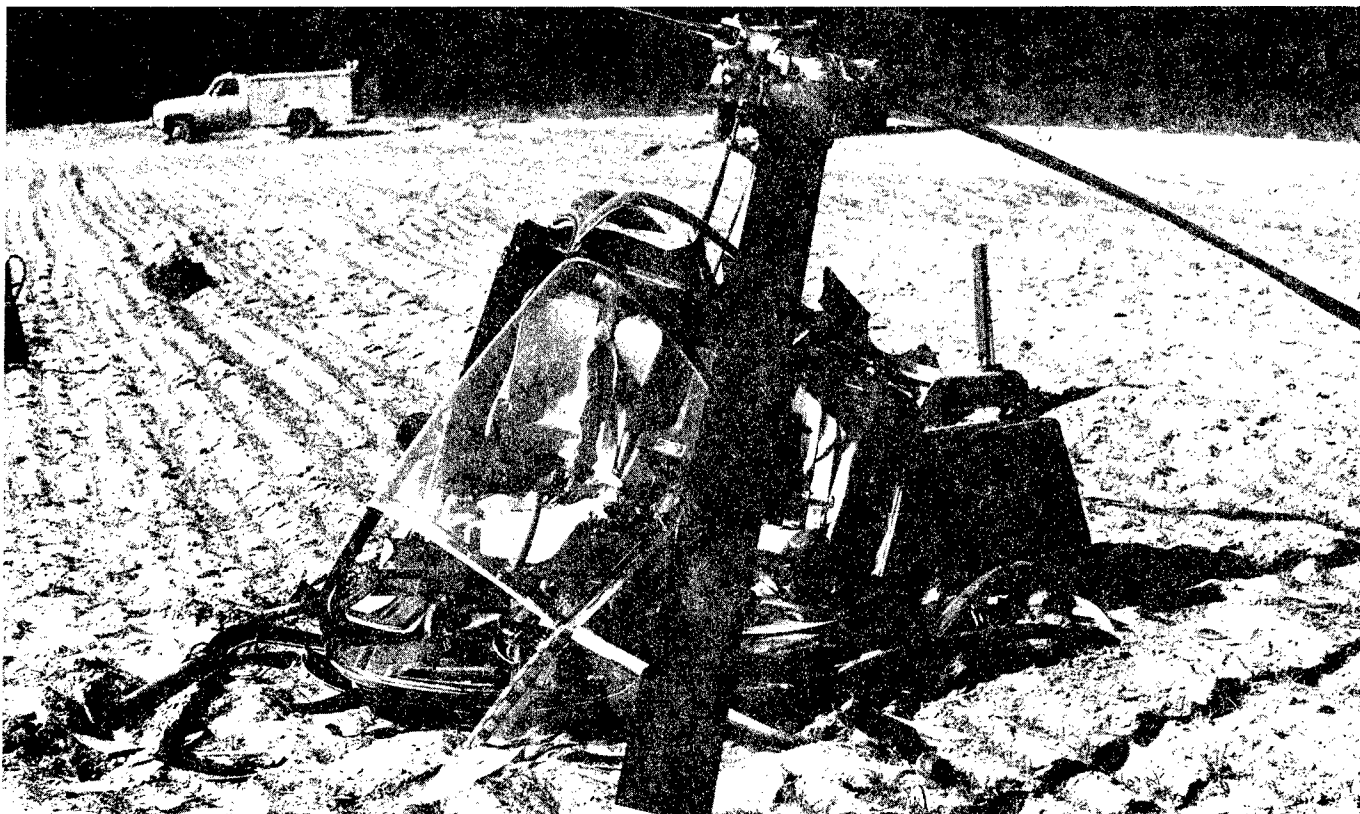
Tail rotor effectiveness was lost when an object hit the tail rotor blade of this TH-55. The student pilot did not follow correct emergency procedures and aircraft crashed.
