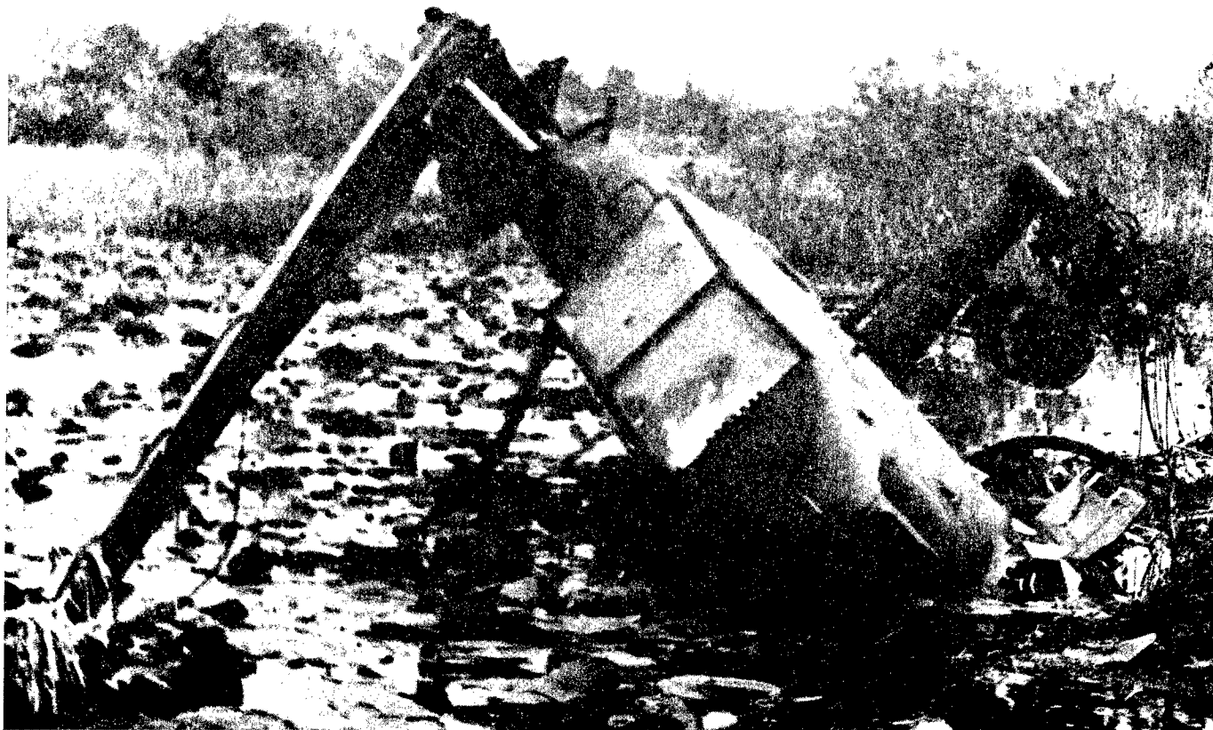
AH-1 main drive shaft failed during flight. Pilot entered autorotation and landed in a marshy area.
