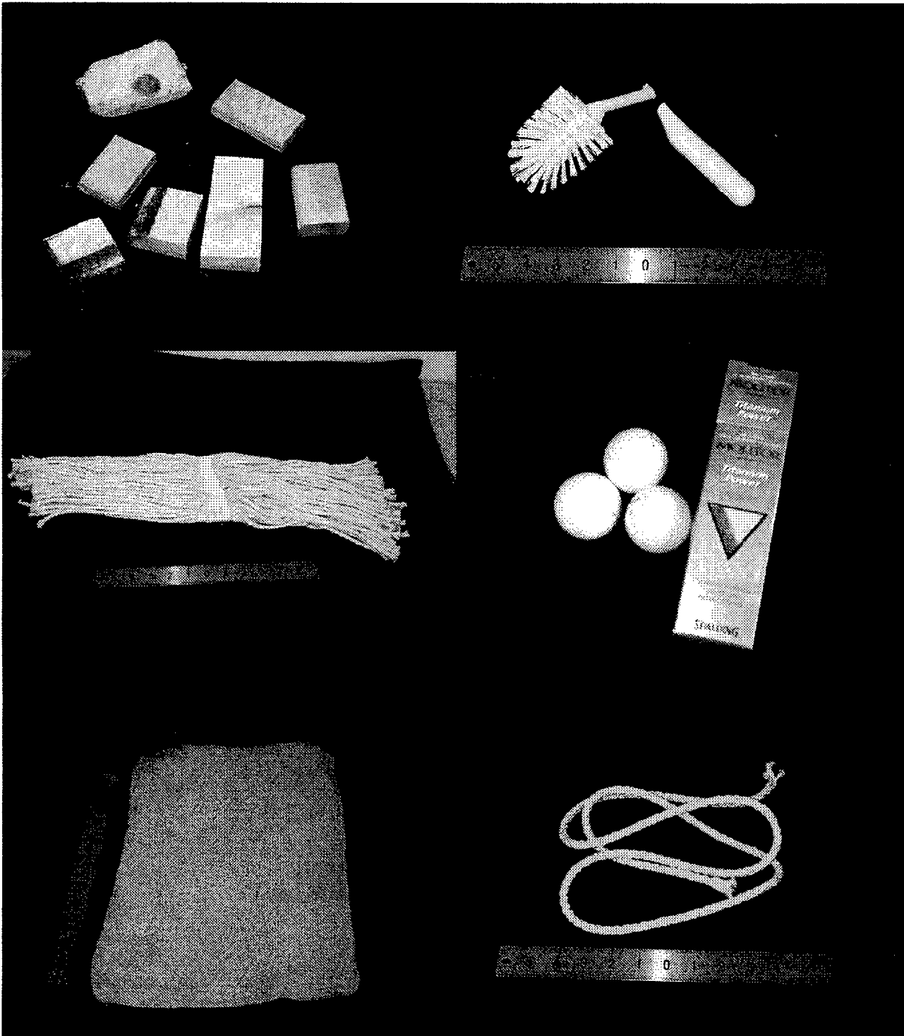
Figure 6. Samples of some items (“solids”) introduced at the pump inlet.
