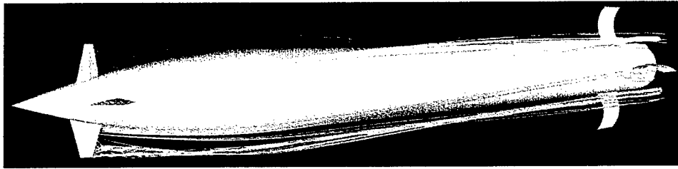
Figure 14a. Particle traces for Mach 1.6, 0° angle of attack.
