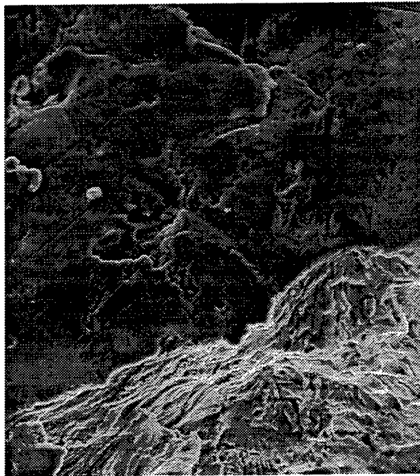
Figure 20. Magnified SEM of Figure 19, Showing Intergranular Attack on the Surface of the Bore Adjacent to the Primary Fracture Origin; Magnification 200 \times .
