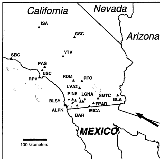
Figure 3. The locations of the 19 broadband, three-component instruments from the TERRAscope and ANZA networks and a temporary network in southern California that form our large aperture array. The thick arrow in the lower right denotes the direction of arrival of the Bolivian event.
