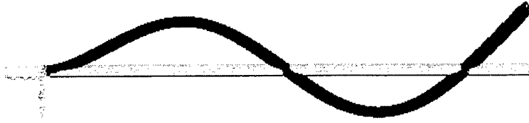
Fig. B-5. Seventh vibrational mode for split-set rock bolt, f_7 = 232 \text{ Hz} .
