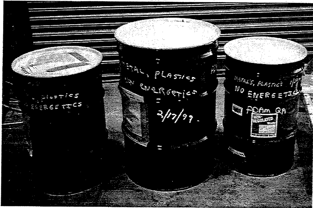
Figure 13 Drums with deactivated debris for shipment to metals recycler
