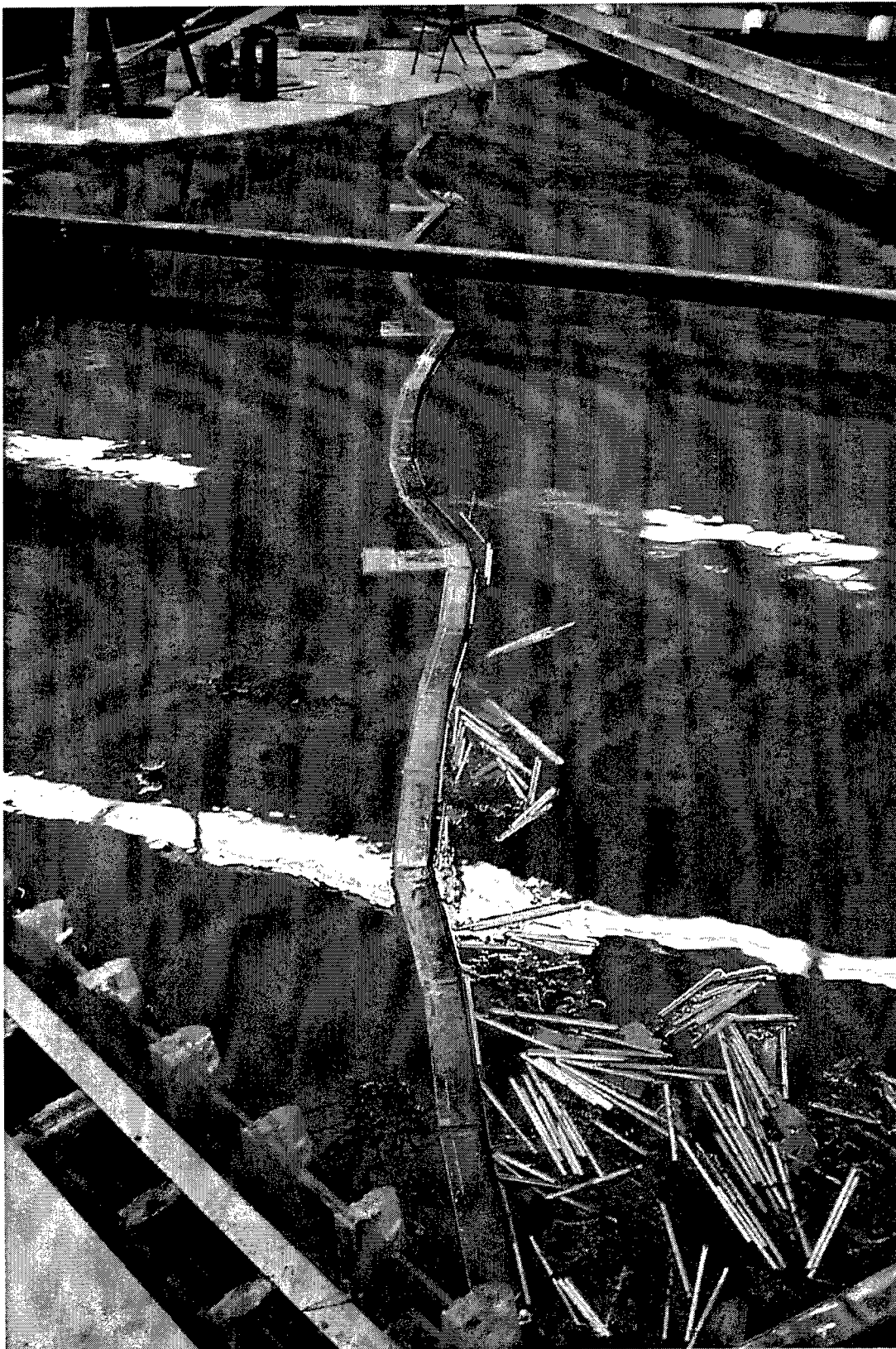
Photo 35. Debris at powerhouse Unit 1 and in Unit 0 sluiceway entrance; final boom alignment; discharge per unit 297.339 cu m/sec (10,500 cfs); pool el 74.5
